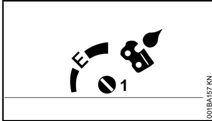
Use the adjusting screw (1) (on underside of machine) to vary the oil feed rate as required.
