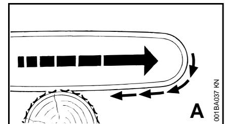
When the chain on the bottom of the bar – overbucking – is suddenly pinched, caught or encounters a foreign object in the wood, the chain saw may suddenly
