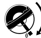
Place the cliplock filler cap (bayonet-type) in position, turn as far as stop and fold the cliplock down.
