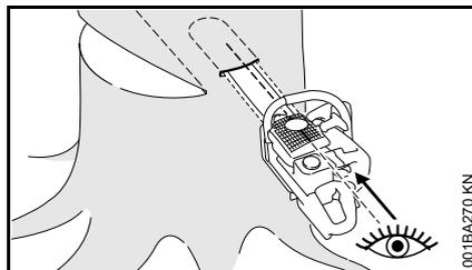
Where possible, use a plunge blade. The plunge blade and the upper/lower side of the guide bar are parallel.
