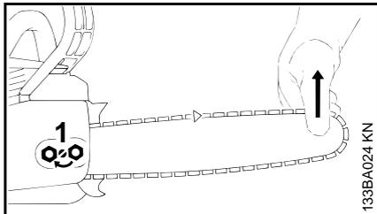
Retensioning during cutting work:
