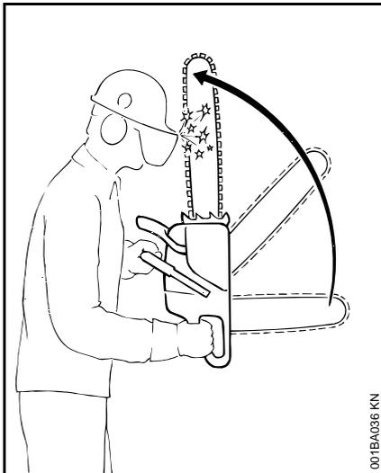
Kickback occurs when the saw is suddenly thrown up and back in an uncontrolled arc towards the operator.
